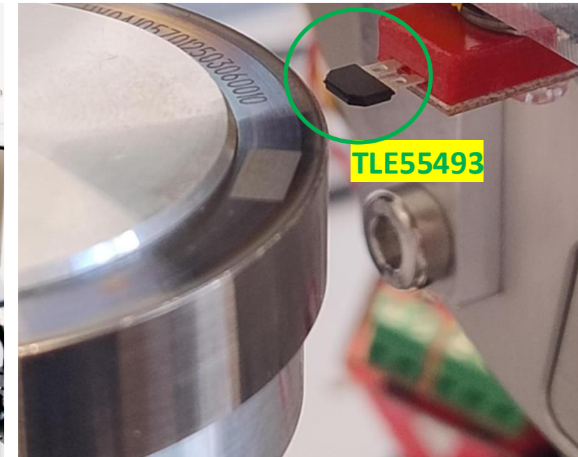
High-End Magnetic Pole Wheel Scanner – automated airgap and rotation sweeps, laser interferometer + wheel marker for alignment.
