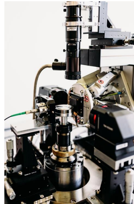
High-End Magnetic Pole Wheel Scanner – automated airgap and rotation sweeps, laser interferometer + wheel marker for alignment.
